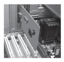
Figure 3. Inserting the PCI Board
